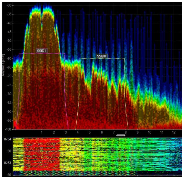
Chanalyzer is designed to bring simplicity and power to the process of wireless troubleshooting. It combines Wi-Spy's ability to read raw RF data with your computer's built-in Wi-Fi card to show you how environmental Wi-Fi saturation and non-Wi-Fi transmitters are affecting your network. Chanalyzer is capable of displaying activity in the 2.4 GHz band, 5 GHz band, or both simultaneously if using Wi-Spy DBx or a Cisco access Point.
