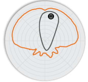
Figure 5. H320 5GHz Elevation Antenna Patterns
