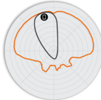
Figure 4. H320 2.4GHz Elevation Antenna Patterns
