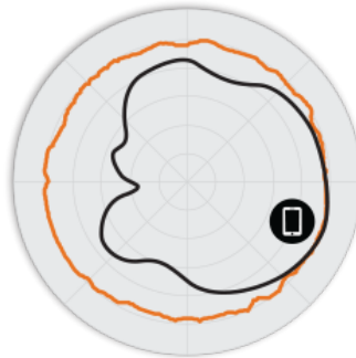
Figure 3. R510 5GHz Azimuth Antenna Patterns
