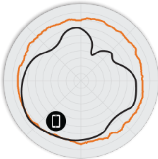
Figure 2. R510 2.4GHz Azimuth Antenna Patterns
