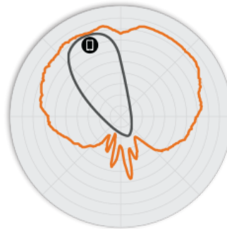
Figure 4. R510 2.4GHz Elevation Antenna Patterns
