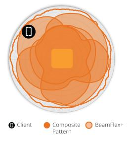
Figure 2. R710 2.4GHz Azimuth Antenna Patterns
