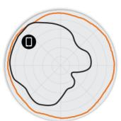
Figure 4. R710 2.4GHz Elevation Antenna Patterns
