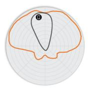
Figure 5. R710 5GHz Elevation Antenna Patterns
