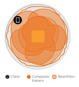
Figure 2. R730 2.4GHz Azimuth Antenna Patterns
