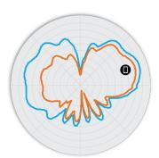
Figure 5. R730 5GHz Elevation Antenna Patterns
