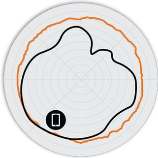
Figure 3. M510 5GHz Azimuth Antenna Patterns
